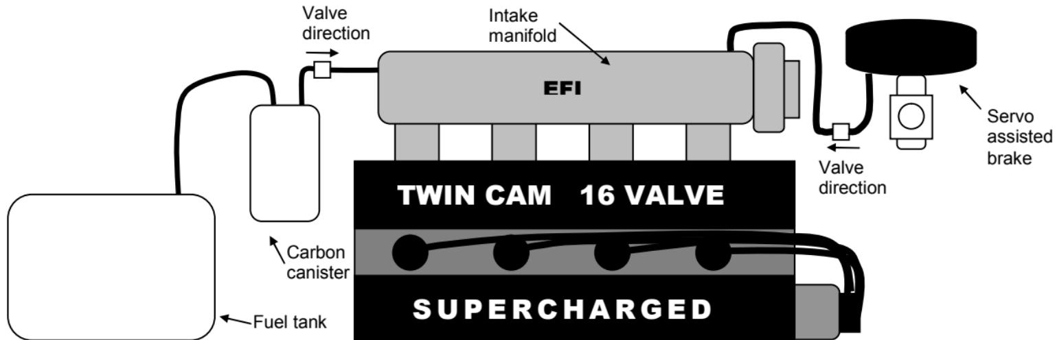
It is imperative that there is an air filter on the inlet of the supercharger. If this is neglected, there is a risk of damage to the supercharger from objects being sucked into the inlet. An open filter arrangement, such as K&N cone filters, will in some cases give induction noise from the impeller. To prevent induction noises please use a closed filter box as seen on most OE applications.
